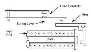
Figure 01: Electromechanical Relay (EMR)
