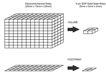
Figure 03: Package Size/Footprint Comparison
