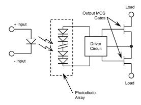
Figure 02: Solid State Relay (SSR)
