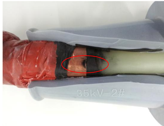
Fig. 5 Fault cable terminal
