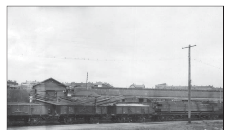
“Newcastle – Railways – Newcastle Railway Yard (September 1927)” Railroad Yard at Newcastle. The three loads shown contain lumber. The car on left (about 16ft long) contains dimension timber. The middle car, logs, and the flat car on right carries hewn hardwood timbers. (SOURCE: NEWCASTLE REGION LIBRARY)
