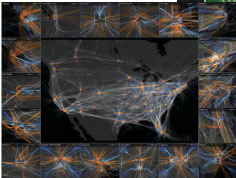
This award-winning image by Sandia researcher Andy Wilson shows PANTHER's geometric and temporal trajectory analyses of air traffic patterns from 43,000 flights over the U.S. on April 4, 2014. White lines represent level flight, orange lines indicate ascent and blue lines show descent.
