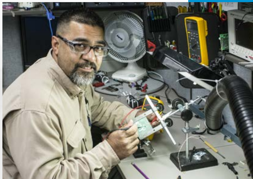
Ben Flores from Pantex Maintenance checks the conductivity of a printed circuit board of an X-ray machine. Learn more about Pantex employees in the special Pantexan feature on page 14.
