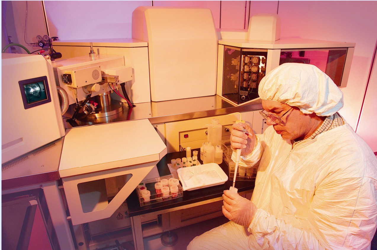
MC ICP-MS system for low-level actinides measurement
