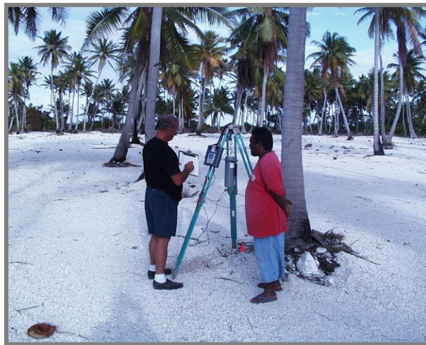
Figure 3. A Surveillance and Measurement System (SAM 975 unit) with a 3'' \times 3'' NaI detector suspended at 1 meter above ground (Rongelap Island, LLNL in-situ gamma survey, April 2001)
