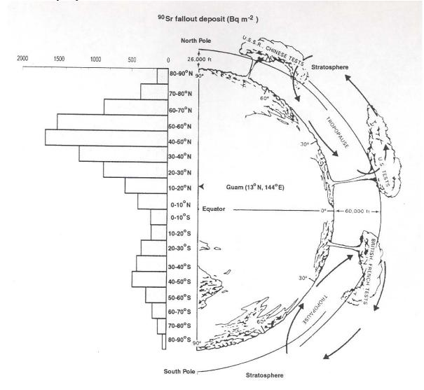
Figure 3. Hemispherical air circulation patterns and associated latitudal <sup>90</sup> Sr deposition densities on earth (modified after Kathren, 1984).
