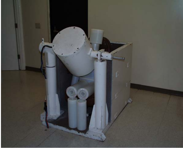
Figure 1. Whole body counting system on Rongelap Island with a plastic calibration phantom sitting in the chair.
