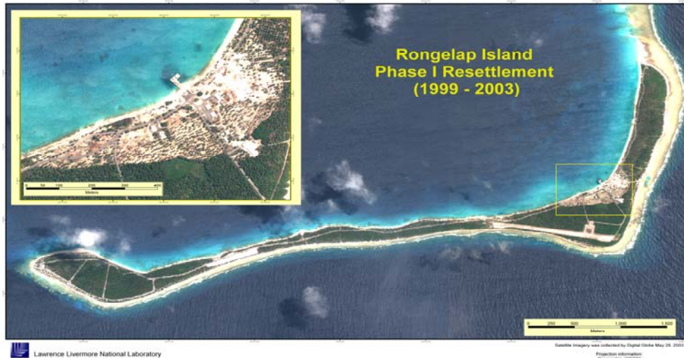
Figure 3. Satellite image of Rongelap Island showing (insert) the location of the community center where surface soil was removed and replaced with clean crushed coral fill (approximately 11.4 ha or 36.1 acres). The initial phase of this work was completed in March 2001. A detailed in-situ gamma monitoring survey of the entire area was conducted in May 2001. The results of this study show that the combination of limited soil removal and addition of crushed coral fill was very effective in reducing the external exposure rates. The clean surface layer of coral also has the added benefit of reducing potential exposures from inhalation and ingestion of plutonium and/or other long-lived radionuclides present in the soil (Hamilton et al. , 2001).
