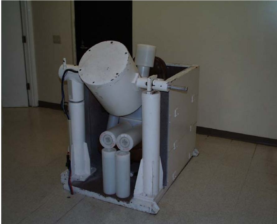
Figure 1. The Rongelap Atoll Massic-Bolton whole body counter based on a design showing a plastic calibration phantom sitting in the chair.
