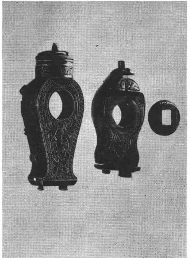
A LATE FORSYTH SCENT BOTTLE MAGAZINE #3084 (LEFT), WITH QUICK RELEASE CATCH ON SIDE, AND FOR COMPARISON A CRUDE FORGERY AT RIGHT.
