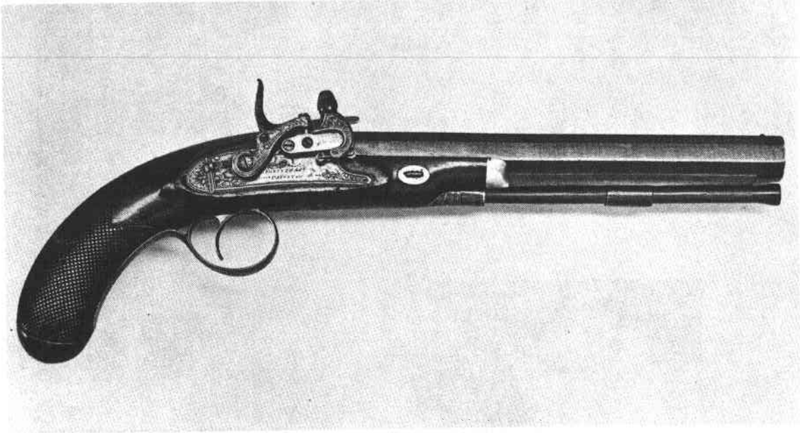
ANOTHER TYPE OF FORSYTH LOCK, THE SLIDING MAGAZINE. THE MAGAZINE BEING ACTUATED BY THE HAMMER.
