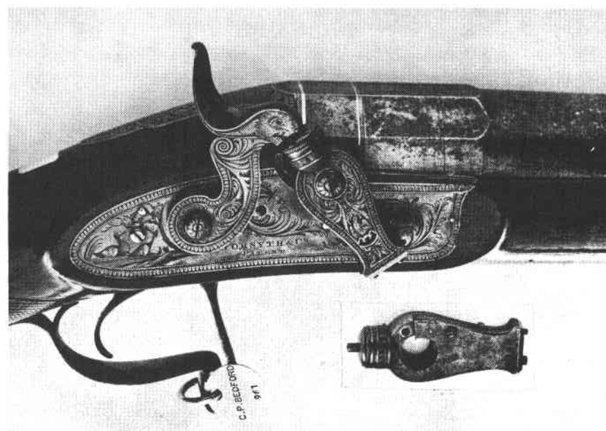
FORSYTH 4 BORE SHOTGUN WITH GENUINE SCENT BOTTLE IGNITION OF LATE TYPE HAVING QUICK TAKE-OFF, ENGRAVED, SCENT BOTTLE. BACK OF REMOVED LOCK ALSO SHOWN.
