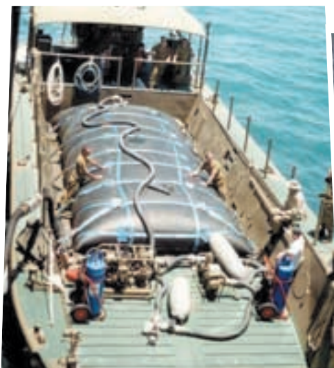
The TFCM inside the welldeck of the LCM8 being filled from a Naval asset
