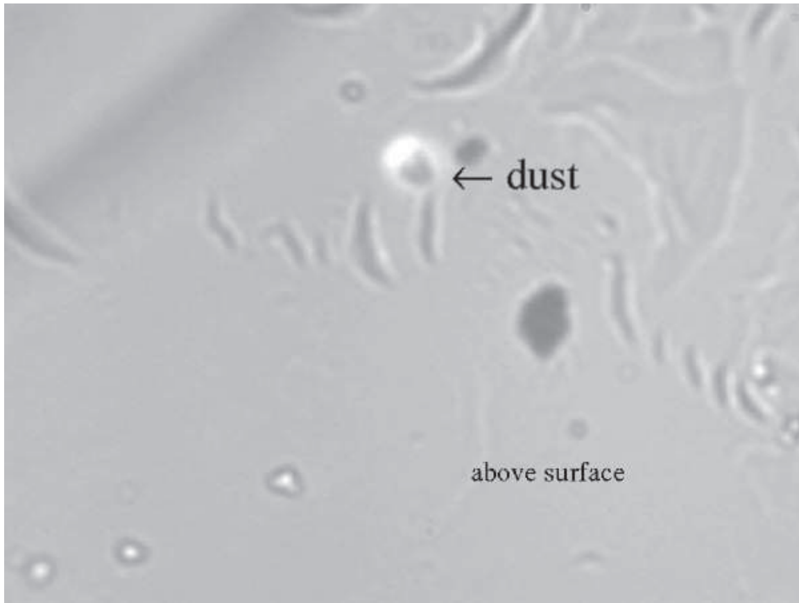
Figure 32: A piece of terrestrial dust is stuck to the surface of the aerogel.
