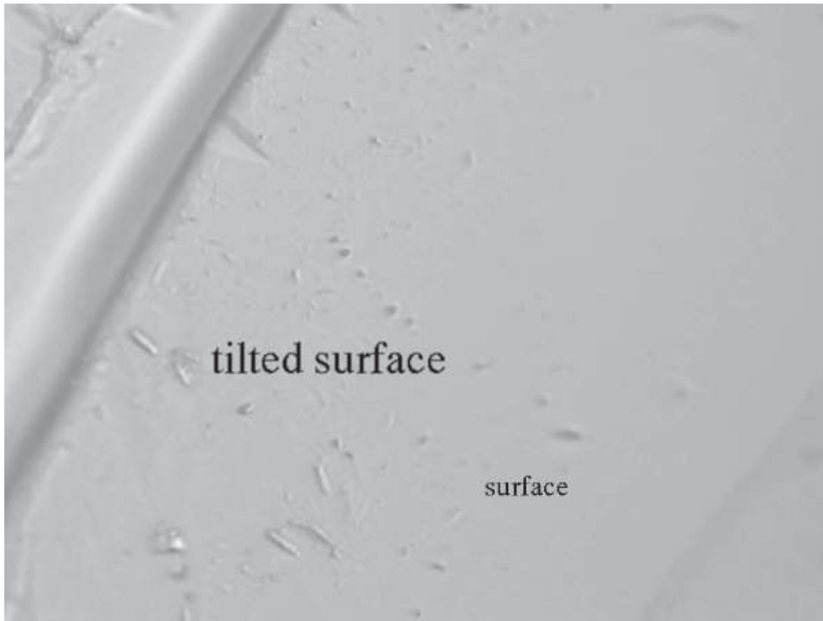
Figure 35: The surface of the aerogel is tilted with respect to the microscope.
