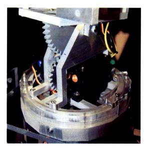
Figure 7-12: Neck servos connected to gears.
