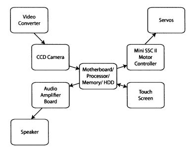
Figure 7-7: Diagram of electronics components in robot.
