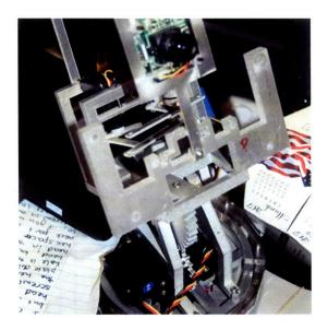
Figure 7-16: An assembled head without eyes.
