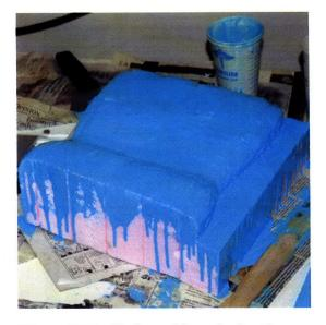
Figure 7-18: Body mold ready for thermoforming.
