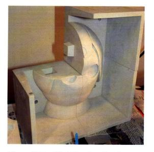
Figure 7-26: Three-fourths of a four-part mold
