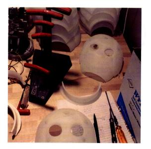
Figure 7-10: Stack of shells waiting to be painted
