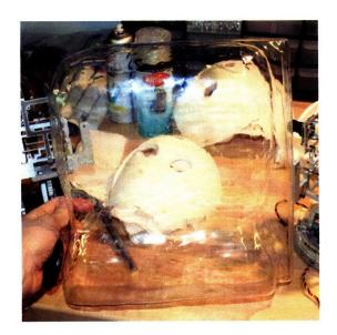
Figure 7-19: Thermoformed body shell before painting.
