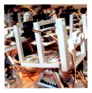
Figure 7-13: Eye servos attached to frame.
