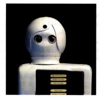
Figure 8-8: Close up of robot's head with camera seen above eyes.
