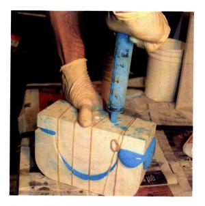
Figure 7-27: Injecting silicone into one mold set.
