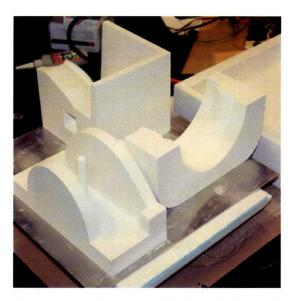
Figure 7-23: Printed molds directly from 3D printer.
