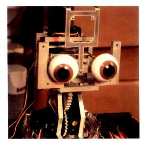
Figure 7-32: Eyes attached to head frame without shell.
