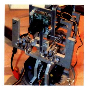
Figure 7-14: Eye attachment mechanism.
