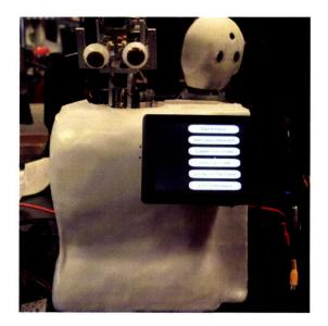
Figure 7-21: Robot with body shells attached.
