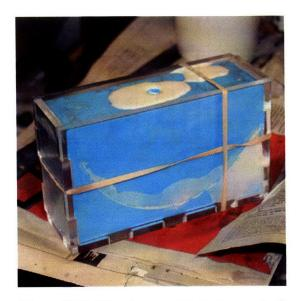
Figure 7-29: Plastic poured into two-part silicone mold.
