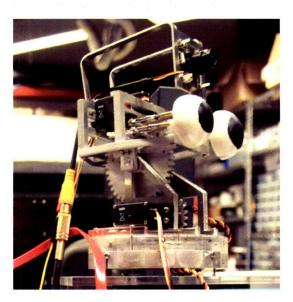
Figure 7-5: Original head design prototype.
