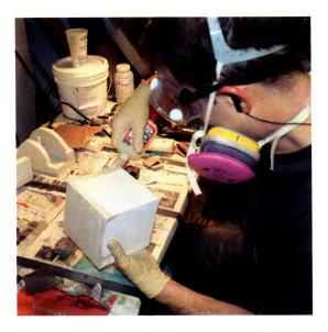
Figure 7-24: Applying cyanoacrylate to harden molds.
