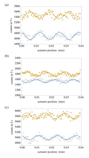
Fig. 5. (Color online) Residual variations in the coincidence counts  $N_{AB}$  ( $\Box$ ) and  $N_{A'B}$  ( $\bullet$ ) for the which-way setting. A sine-squared fit has been applied by hand. The periodic variations match the period of the interference fringes, indicating remaining phase information. The fluctuations about those variations are dominated by Poisson counting noise. As in Fig. 4, the rows indicate: (a) no delay, (b) free-space delay, and (c) fiber delay.
