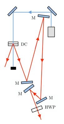
Fig. 3. (Color online) Schematic of the free-space delay in the idler arm. Only the relevant components are shown. Four mirrors (M) are used to elongate the optical path traveled by the idler photon between the downconversion crystal (DC) and the half-wave plate (HWP) selecting the measurement basis.
