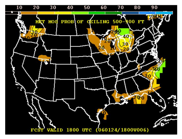
*Figure 2.* MOS also can be viewed graphically in many ways, including this chart which indicates the probability of a ceiling of 500 ft to 900 ft AGL valid at 1800 UTC on January 24.
