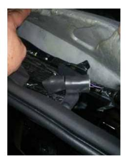
Place the connectors back down into the harness bundle as shown.
