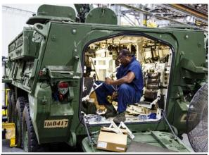
An Anniston Army Depot employee works on installing new internal parts on a Stryker.
