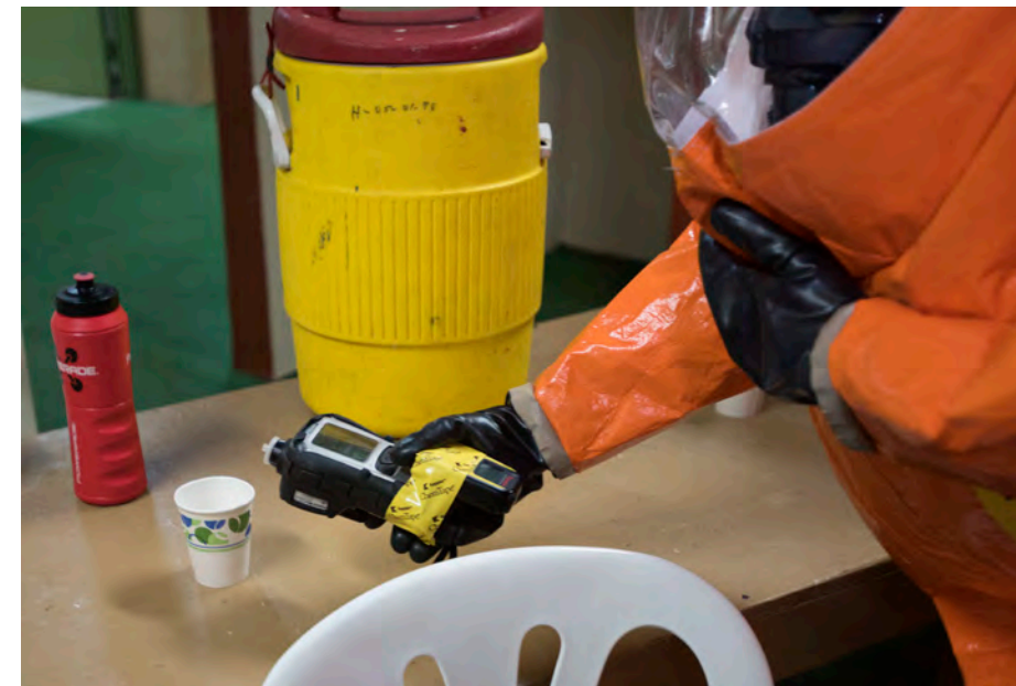
U.S. Army Sgt. Darwin Jurentkuff, survey team member, uses a MultiRAE Pro and RadEye to check for toxic chemicals and radiation.
