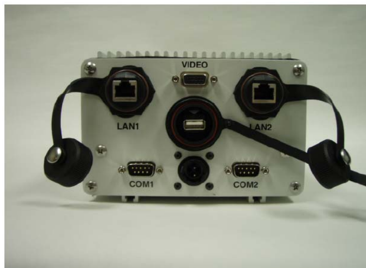
Figure 10.10 MCNU Interface Panel
