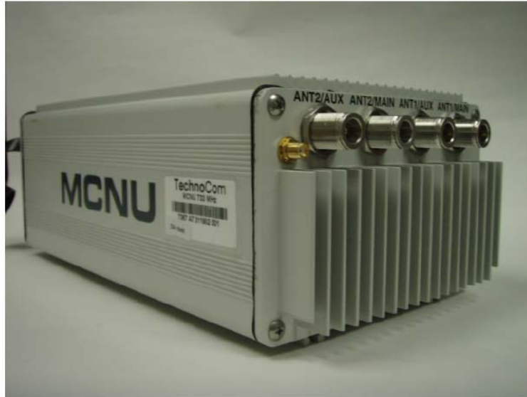
Figure 10.11 MCNU RF Panel
