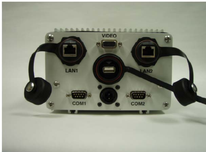
Figure 6. MCNU Interface Panel
