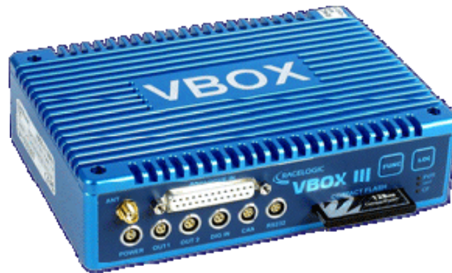
Figure 10.7 VBOX III GPS Data Logger
