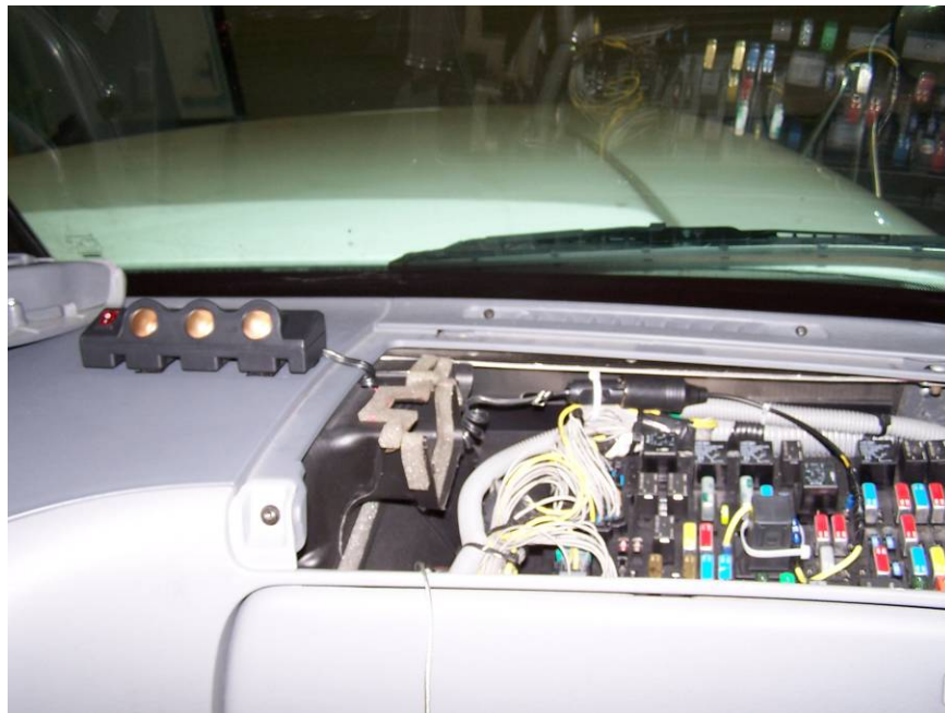
Figure 11.7 Dash Access to DC Power and J-1708
