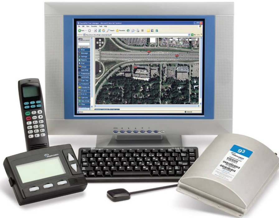
Figure 5. PeopleNet OBC and Display Used in the WRI POC
