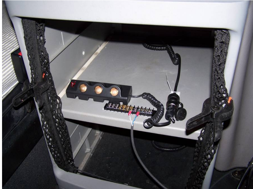
Figure 11.6 Sleeper Berth DC Power and J-1708 Access
