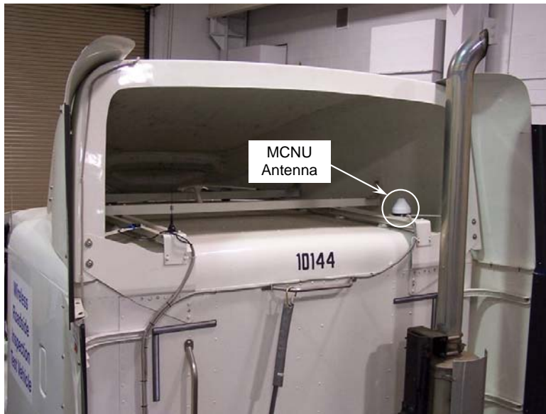
Figure 22. Placement of the MCNU Dome Antenna on WRI Test Truck
