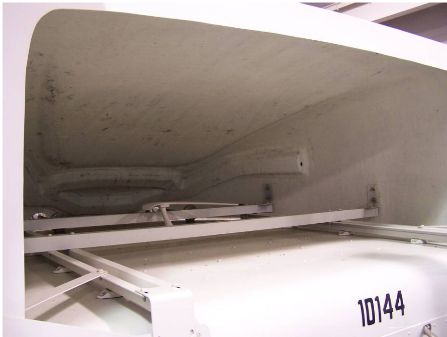
Figure 11.7 Air Fairing Support Structure for Antenna Placement
