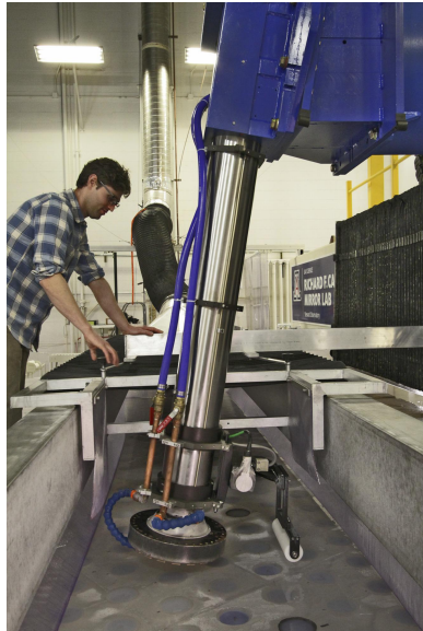
Figure 6. LOG spindle in position to generate the rear surface of Segment 3.
