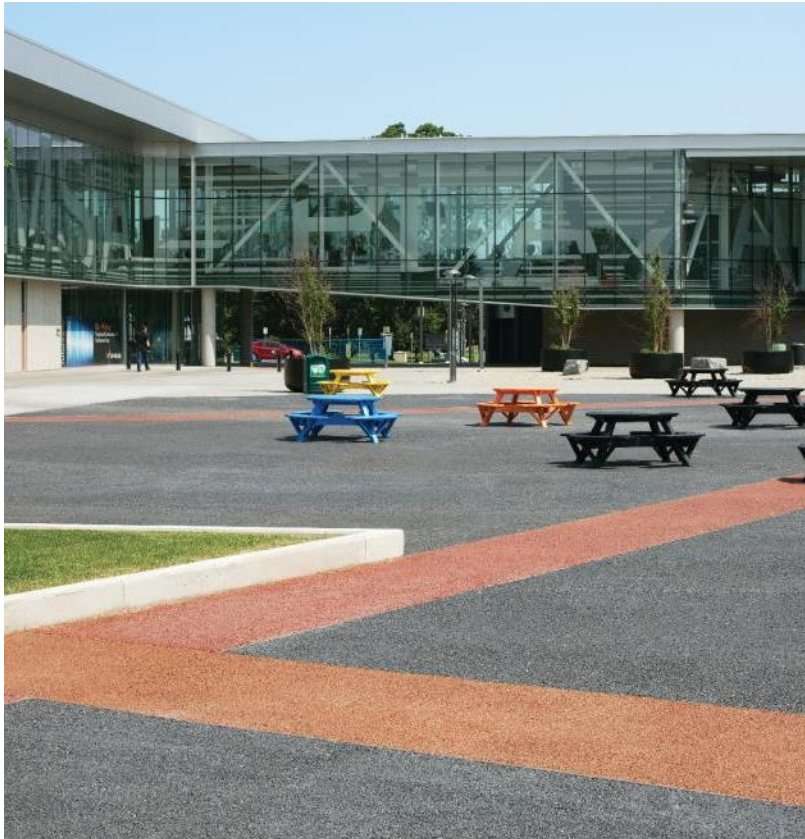
Hamilton, Canada: pervious concrete Hydromedia™ - absorbing the rainwater and facilitating natural flow in the soil - was used to shape the forecourt of Mohawk College in Hamilton, Canada.
