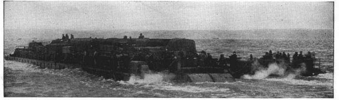
FLOATING HIGHWAYS: Powered by twin outboard motors, a Rhino Ferry loaded with men and supplies heads for an Allied-held beach. These self-propelled
