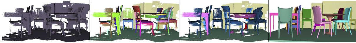
Figure 17: From the incomplete and cluttered scan on the left, the approach of [NXS12] first oversegments the point cloud (mid-left), then iteratively merges segments which agree on class labels (mid-right), and finally deforms a set of detected models to best resemble their segmented objects (right).
