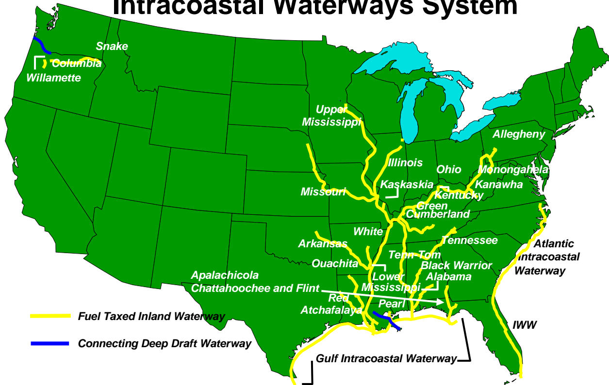
Figure 1-1. The Fuel-Taxed Inland and Intracoastal Waterways System
