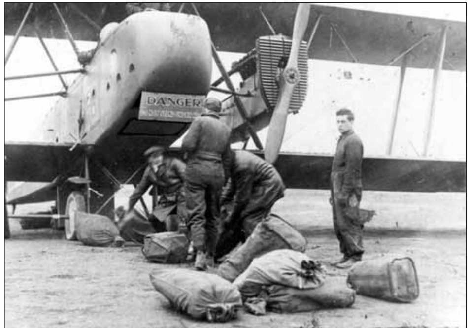
Heller Field was located in Newark’s North Ward and was in operation from December 1919 to May 1921 as a U.S. Mail airfield. Here, mail bags are dropped from wells in the forward part of the fuselage.
