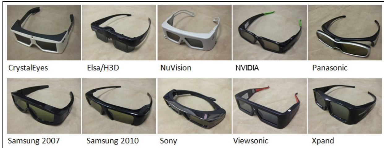
Figure 1: Ten of the eleven active shutter glasses tested in this study: (a) StereoGraphics CrystaleEyes CE-1, (b) ELSA/H3D, (c) NuVision 60GX, (d) NVIDIA 3D Vision, (e) Panasonic TY-EW3D10U, (f) Samsung 2007, (g) Samsung (2010) SSG-2100AB, (h) Sony TDG-BR100, (i) Viewsonic PGD-150 DLP Link, and (j) Xpand X103 Universal. Sharp AN3DG10 not shown.
