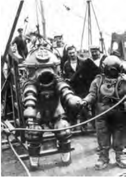
Diver Jim Jarret inside the Tritonia ADS (left) during the 1935 exploration of the wreck of RMS Luisitania at 312 feet.
