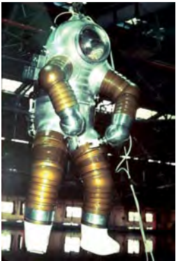
The SAM suit is a lighter, more anthropomorphic version of the JIM suit. It features one large viewport compared to JIM's four small ones.
