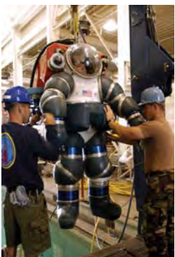
The Hardsuit 2000 is part of the Navy's new Submarine Rescue Diving and Recompression System implemented in 2008. The ADS is used to examine downed submarines and clear their escape hatches before the rescue effort begins.
