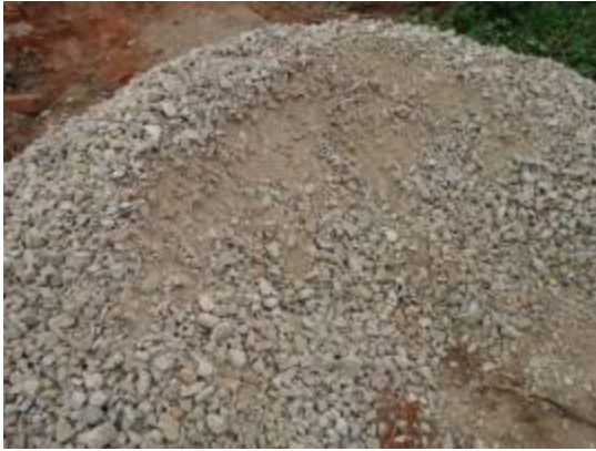
L-R: Poor quality aggregates dominated by dust that was used for Plain Concrete Cement (PCC); Completed PCC works in Lwela-Masaka
