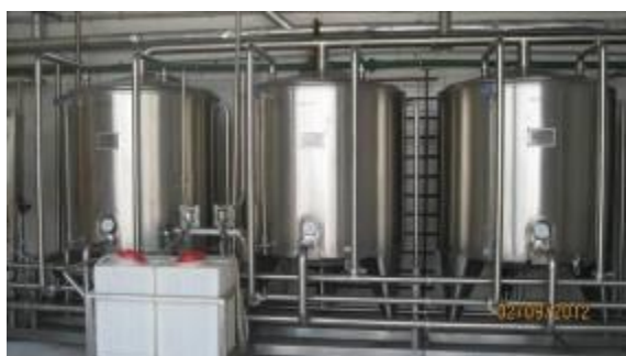
Left: Cleaning system tanks Right: Packed milk ready for export
