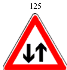
Oncoming Traffic. Posted where oncoming traffic normally is not expected (for example, autobahns, and construction sites).
