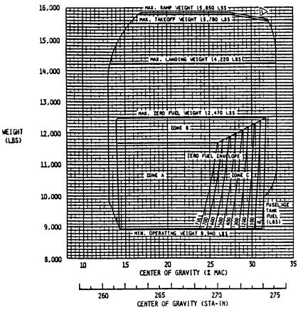
Wheel Loading Limit Line - Reduce Maximum Ramp Weight (15, 850 lbs.) by 50 Lbs. of wing fuel for each percentage of MAC aft of 27.5%.
