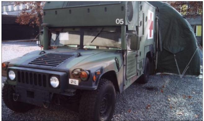
The Chemically and Biologically Protected Shelter uses an expanded capacity Humvee and a hardwalled lightweight multipurpose shelter attached to the bed of the Humvee.
