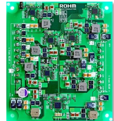
Avnet Inc. Power module board (Kintex-7) for Mini-Module Plus development system
