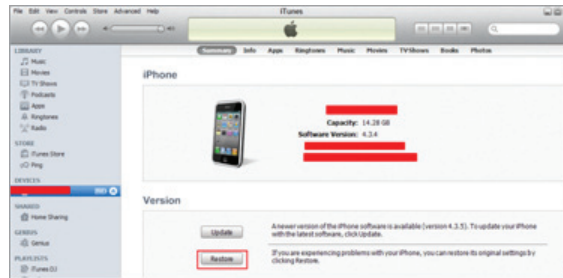
Figure 13. The Restore option in iTunes to reset the phone to its original state.
