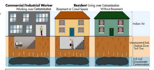
Contamination in the soil and groundwater can take the form of a vapor and travel through soil, entering indoor air through leaks in parts of buildings which are below-around, like basements and crawl spaces.
