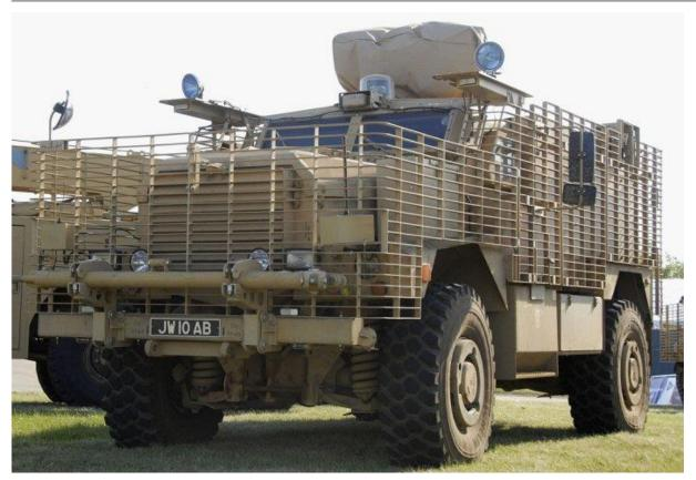
Aware of mobility limitations, in 2010 the MoD evaluated two possible suspension upgrades for UK MRAPs and Ridgbacks were fitted with Oshkosh's TAK-4 (shown) and a Ricardo-engineered revised parabolic leaf spring set-up. (Shaun C Connors)
