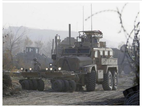
The USMC will retain 2,510 MRAP in two variants including the GDLS-FP's Cougar; this Cougar CAT II 6x6 is fitted with Oshkosh's TAK-4 independent suspension upgrade. (US DoD)
