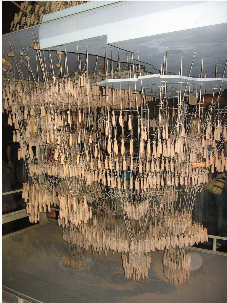
Figure 19: Frei Otto's reconstruction of Gaudí's hanging model for the cripta de la Colònia Güell
