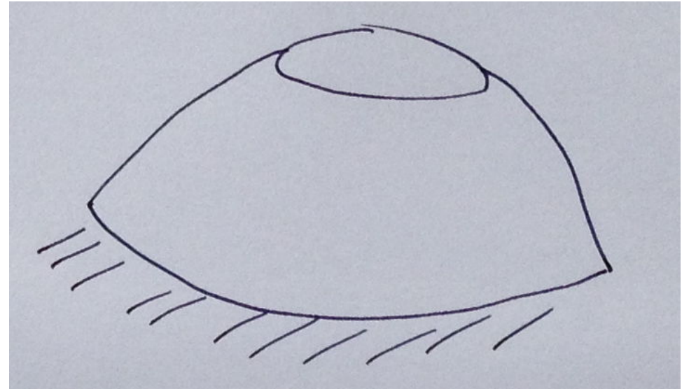
Figure 14: Dome with hole: positive Gaussian curvature, a mechanism, inextensional deformation possible
