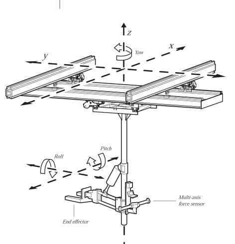
Figure 2: Z-Lift with in-line handle
