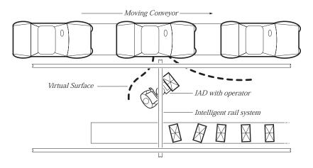
impact with the painted surfaces or interior trim. The system also provides line tracking, or synchronization, in order to keep the virtual window lined up with the moving vehicle.
