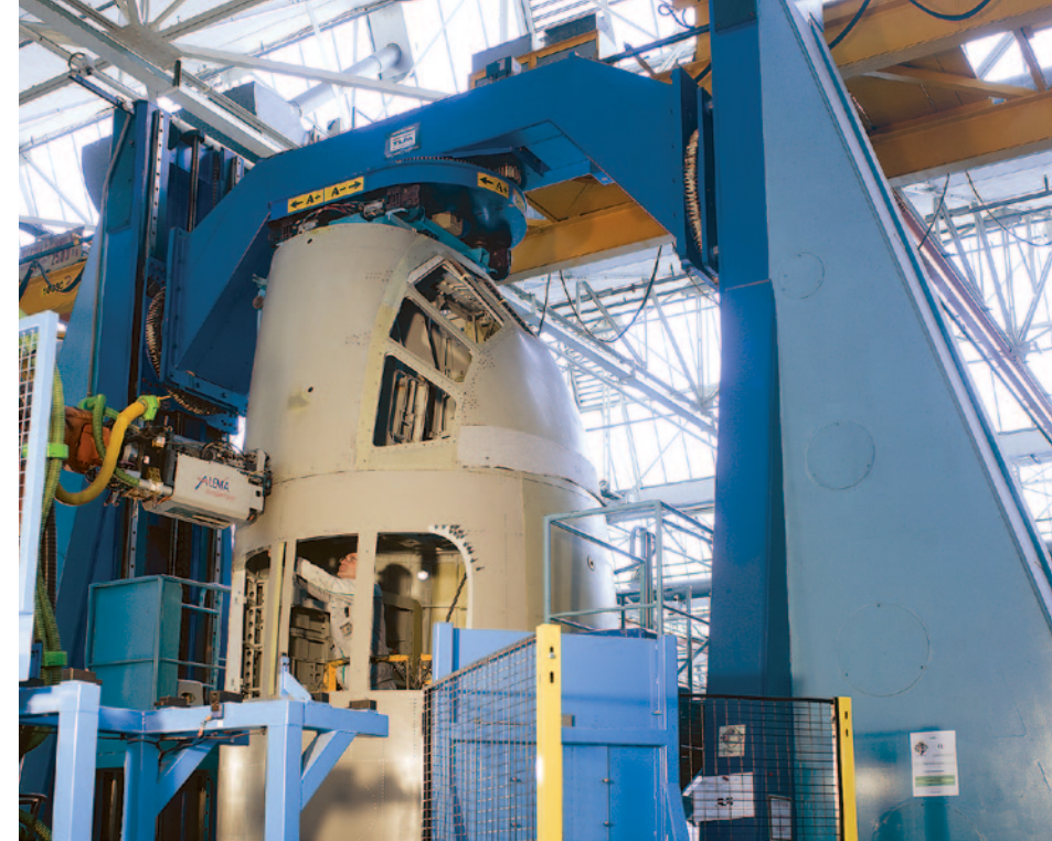
The pressurized section of the Falcon 2000S is circular for structural efficiency under pressurization loads.
