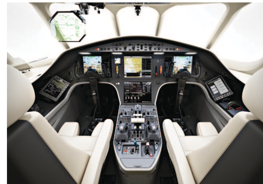
The Falcon 2000S Honeywell EASy II flight deck will have a basic runway performance calculator that will compute V speeds and runway distances.
