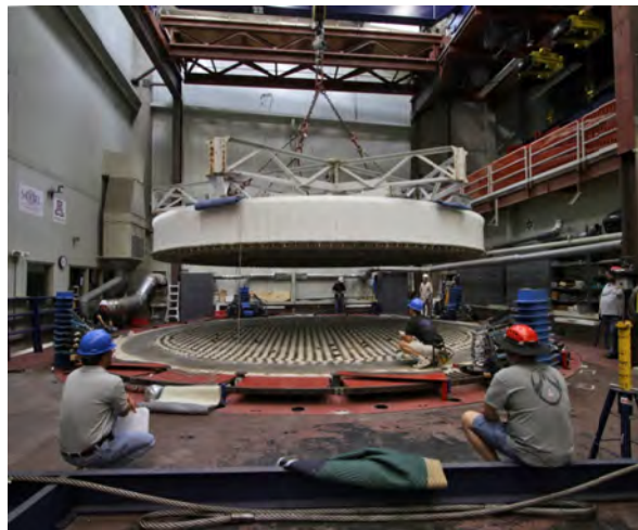
Figure 5 Lifting GMT2 off the casting furnace (19 June 2012)
