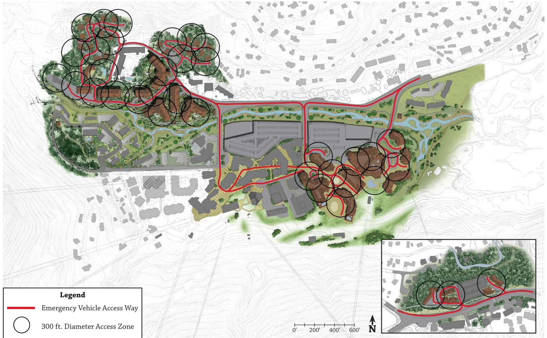
FIGURE 5.18—EMERGENCY VEHICLE ACCESS
