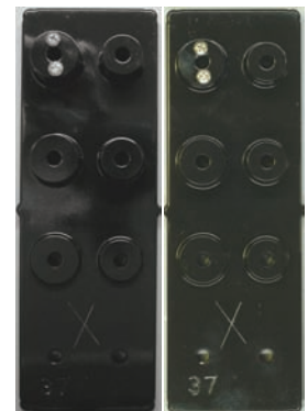
Before After I) Urethane Resin E-Coat
