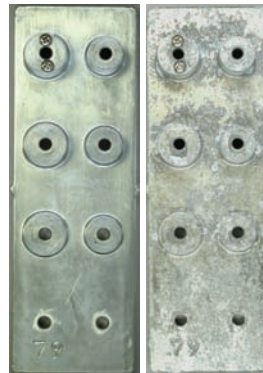
Before After C) Zn Plate, Trivalent Chrome + sealer
