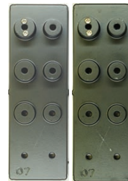
Before After H) Powder Epoxy
