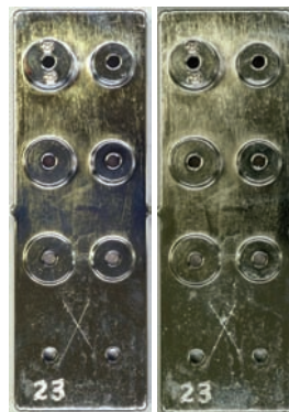
Before After G) Cu-Ni-Cr Electroplate
