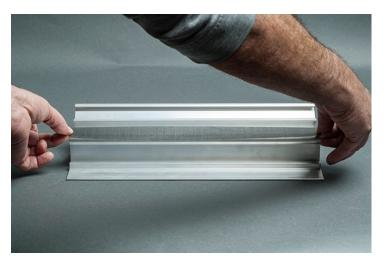
Apply the loop tape to each loop. On the lower loop, center the tape on the top of the loop then slowly slide your finger back and forth over the tape as you slowly work your way to the back edge of the tape. Then continue back and forth from the center and work you way to the front edge of the tape. The objective is to apply the tape without creating any ridges or bubbles on the
