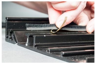
Find the Key Felt in the box that held the keys and hammers. starting at the far right side of the chassis, install the felt by removing the paper backing and applying it to the white key stop. Repeat for the black key stop. Continue applying felt across the keyboard. The felt should end about 4 inches from the left side of the keyboard
