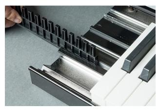
The Riser is a long slat that slides under the key guides to push them up, engaging the keys. Slide the Riser into the same channel under the Key Guides, gently shaking the riser so that the Key Guide stems rise to engage the keys.
