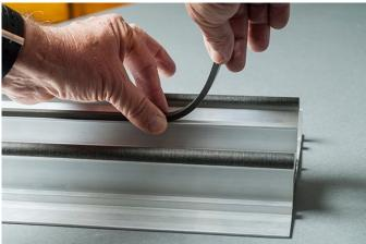
On some early units, this has already been installed. If not, remove the paper backing and apply it to the key rest as shown.
