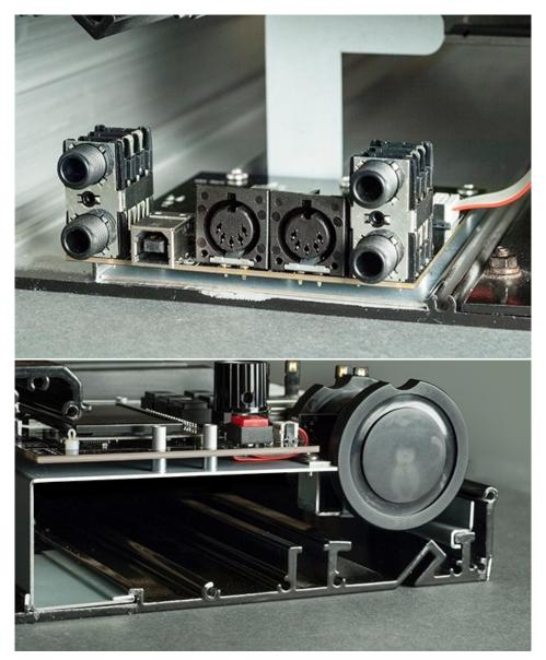
Slide the Main PCB plate into position as shown into slots on chassis rails. BE CAREFUL to align the card edge connector on the Main PCB with the connectors on the last Sensor PCB
