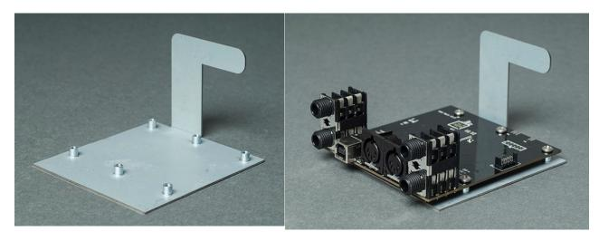
Use six #6 screws to attach the PCB to the plate
