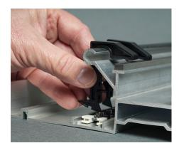
Remove the Hammers from the box and attach elastomer tubing. Carefully slide the hammers onto the top loop.
