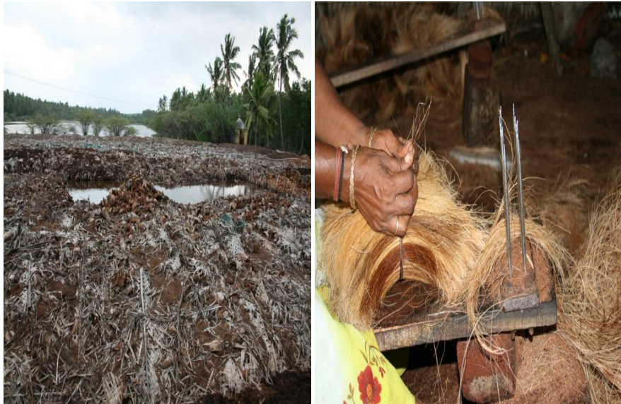
Figure 16 - Traditional production of coir fibre. A: Coconut husks soaked in water on the edge of a lagoon. B: Retted husks are beaten and combed to produce golden fibre and bristle fibre.
