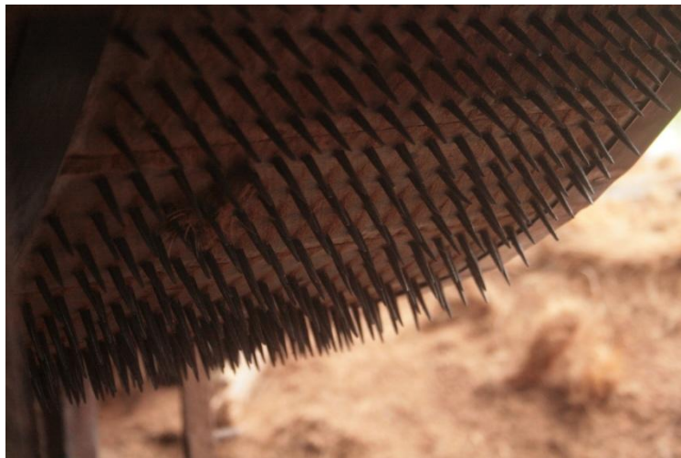
Figure 20 . Needle drum used for fibre extraction. Most found without guards to protect the workforce who hand-feed these machines with retted coconut husks.
