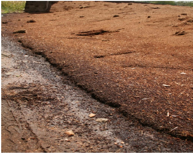
Figure 13 – An example of coir pith washing where the run-off is allowed to contaminate underlying soil. Better practices were seen where the washing process occurred on concrete surfaces, where the run-off was collected and where the run-off was treated.
