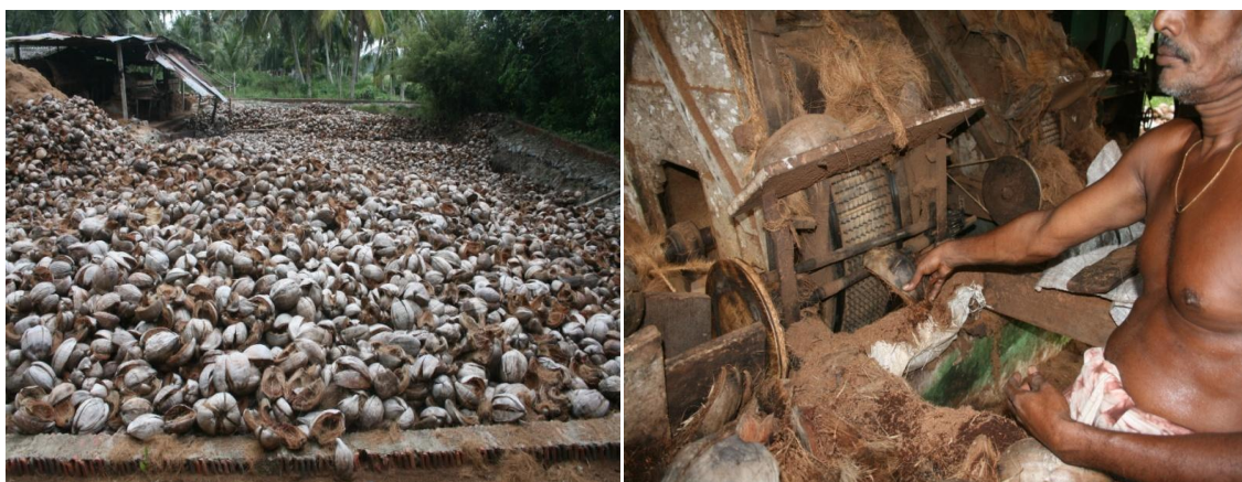
Figure 18 – Husks soaking in a tank and then fed by hand into a machine which is located in the shack in the first photograph, to remove the fibre.
