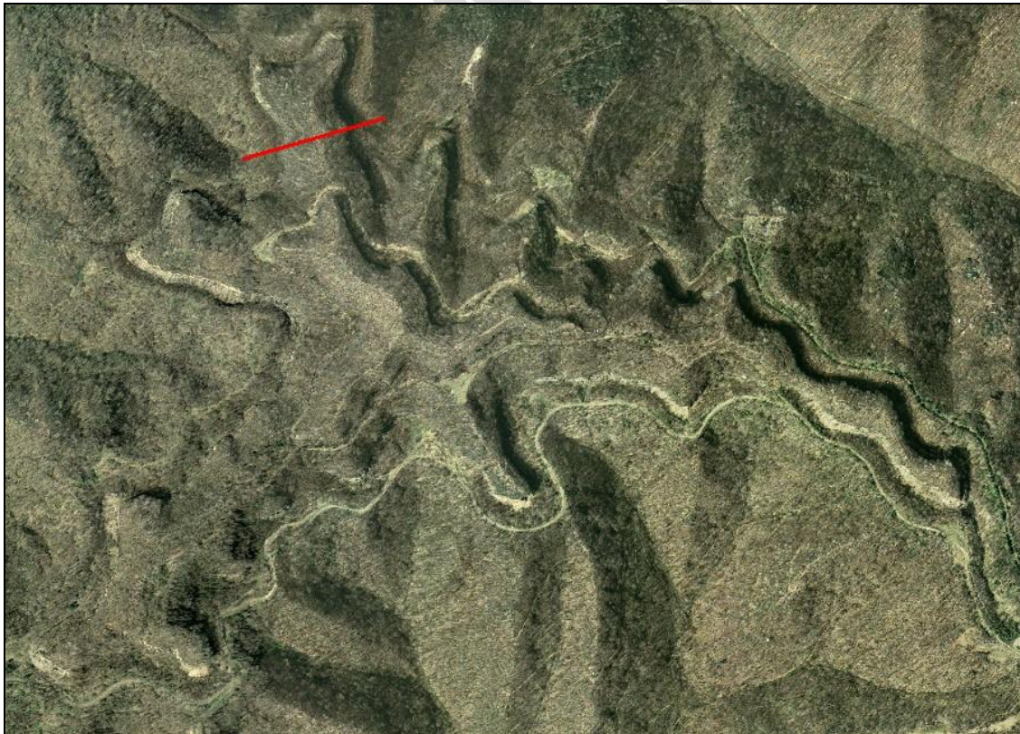
Figure 3. Aerial photograph of auger mining in within the study area.
