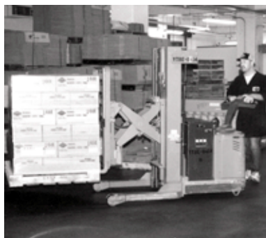
A powered pallet truck is used to transport materials.
