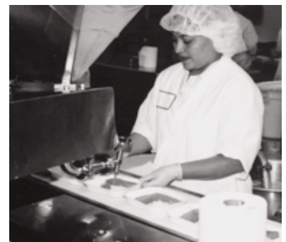
Liquid food dispenser is operated by a hand lever.
