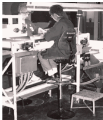
For employees who sit for long periods of time, footrests reduce the pressure behind the knees.
