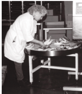
A work surface that is too low requires the worker to stoop.
