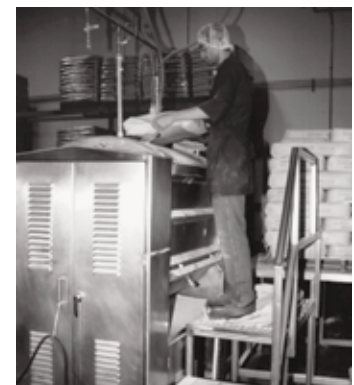
A raised platform allows work to be performed at waist height.
