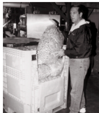
Awkward bending can be prevented by using bins that open from the side.
