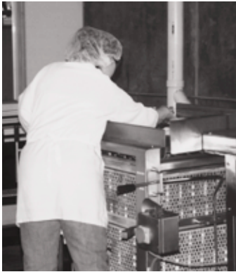
A work surface that is too deep for the worker requires reaching across.
