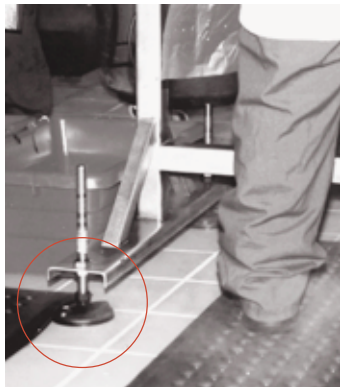
Workstations with adjustable feet can be raised or lowered to fit the worker and the task and prevent awkward postures.
