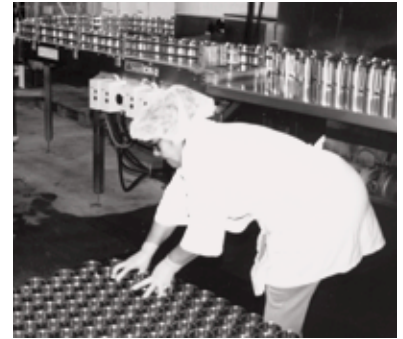
Repetitive gripping with forceful exertions exposes the worker to injury.
