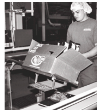
A tilted container provides the worker with easy access to the contents of the container.
