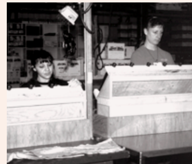
The addition or removal of a platform allows the height of the work surface to be adjusted to fit each worker.
