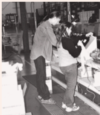
When all employees are expected to work at the same height, some will work in awkward postures.
