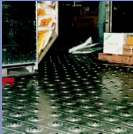
Figure 5.6 A “roller-ball” floor (in a road freight terminal) that allows easy manual moving of airline-type containers, in preparation for loading (the spacing of the roller-balls helps people to walk safely on this type of floor).
