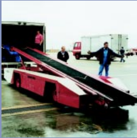
Figure 9.5 A mobile, adjustable conveyor vehicle used at airport terminals to aid loading and unloading goods from trucks.
