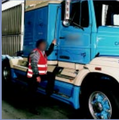
Figure 3.8 Very good steps for access to the cab and other parts of the vehicle.
