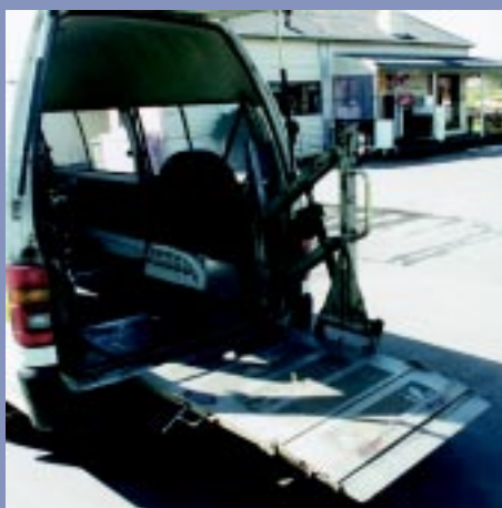
Figure 9.4 A specialised van for transporting people with disabilities and their wheelchairs. The fold-away rear lifter eliminates manual handling of the loaded wheelchairs.
