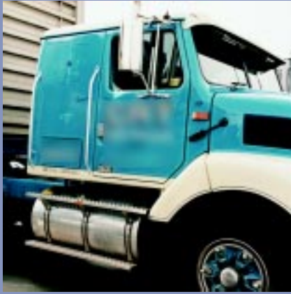
Figure 3.7 Better access steps and grab handles.
