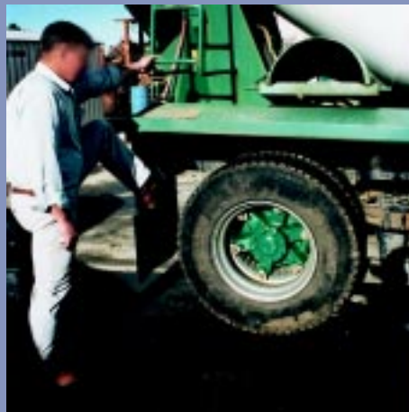
Figure 4.1 Access to rear of concrete mixer is inadequate. The first step is too high and too small, the rung ladder could be improved by increasing the width and using larger bars.
