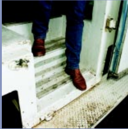
Figures 4.2 and 4.3 The rear access steps to a van, which though good in principle, are in fact hazardous due to poor design. The too narrow bottom step presents a high risk of slipping particularly whilst exiting carrying goods (wet weather would increase the slipping risk).
