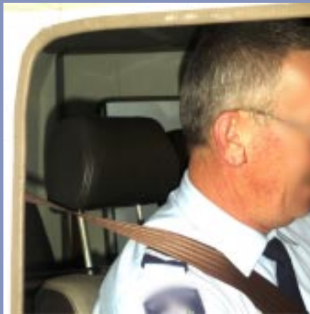
Figure 3.4 A well-designed head restraint is essential in any professional vehicle, as this will decrease the likelihood of a whip-lash injury.
