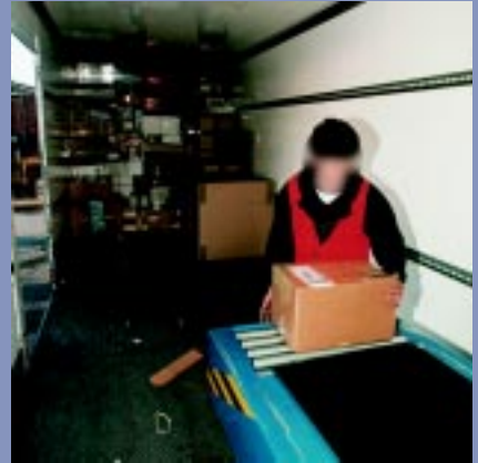
Figures 5.3 and 5.4 A 'Longreach' telescopic conveyor is used to load cargo into a semi-trailer. The conveyor length can be easily adjusted by the operator handling the cargo, as the loading progresses.
