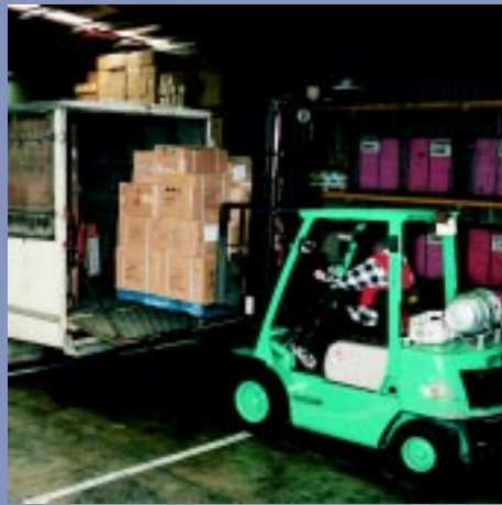
Figure 7.1 A forklift loading a van that is isolated from pedestrian personnel.
