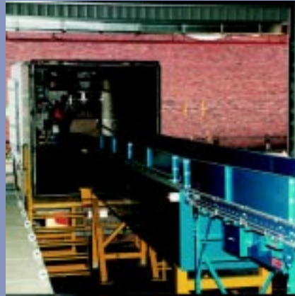
Figures 5.3 and 5.4 A 'Longreach' telescopic conveyor is used to load cargo into a semi-trailer. The conveyor length can be easily adjusted by the operator handling the cargo, as the loading progresses.
