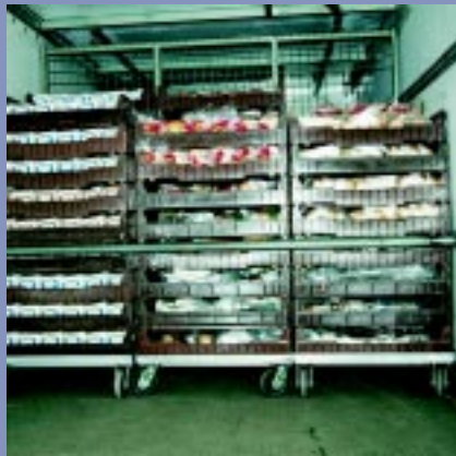
Figure 5.1 A well-organised customised cargo hold for handling 'palletised' loads. Note the easily movable gate is hinged on the side and also runs on a track mounted on the van's ceiling.
