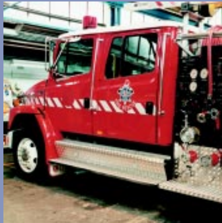
Figure 9.7(a) The general purpose pumper is an excellent example of a vehicle that has been specially developed and designed to address both operational and safety issues. Note the very good access steps and long grab handles. The long grab handles (outside and inside the vehicle) allow a continuous grip to be maintained during entering and exiting of the vehicle.
