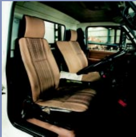
Figure 3.1 Very basic operator seating that lacks adjustment capabilities.
