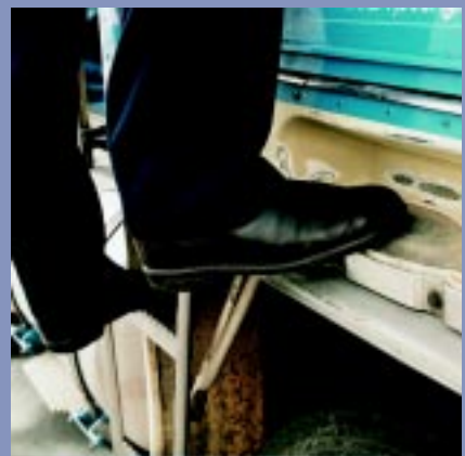
Figures 3.5 and 3.6 The access ladder and step for a cab over design. Although this is an improvement over the single bar rung ladder from earlier models it suffers from very narrow rungs and a well-worn step under the door (potentially quite slippery, particularly when wet).
