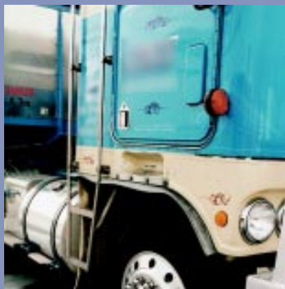
Figures 3.5 and 3.6 The access ladder and step for a cab over design. Although this is an improvement over the single bar rung ladder from earlier models it suffers from very narrow rungs and a well-worn step under the door (potentially quite slippery, particularly when wet).
