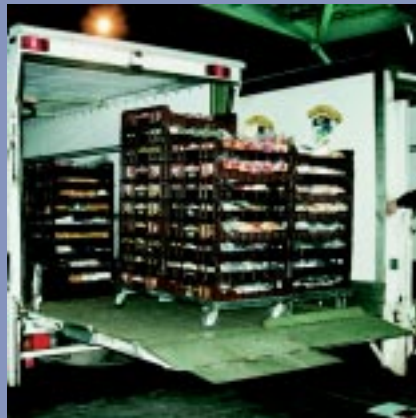
Figure 5.2 A tailgate loader used to move the trolley mounted into the cargo hold.
