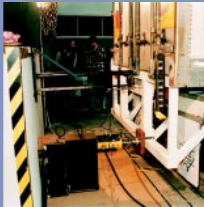
Figure 10.1 View of a well designed rear underrun barrier on a semi-trailer. The barrier shown is under test.
