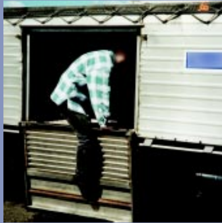
Figure 4.6 The side door opening to a van used for handling newsprint and magazines. In this case the issue of access and good ergonomics for the operator has essentially been ignored.
