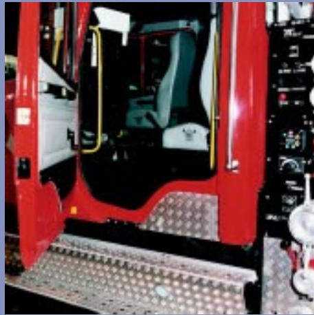
Figure 9.7(b) Interior view of the MFESB vehicle showing good steps, long grab handles and well-designed seats with high backrests and headrests (the seats are designed to hold a fireman's oxygen tanks and allow a quick exit from the vehicle).
