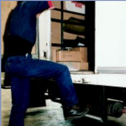
Figures 4.4 and 4.5 These photographs illustrate inadequate, but typical steps and grab handles provided for access to vans. Note the effort required to enter the doorway. Exiting is even more difficult.
