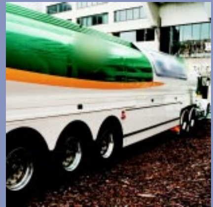
Figure 10.2 An example of a well-designed side skirt on a petrol tanker.
