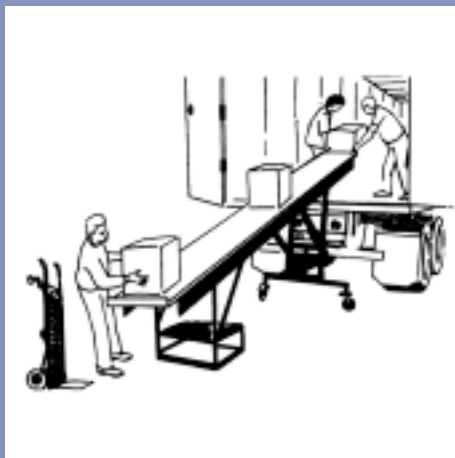
Figure 5.10 A portable, height adjustable conveyor can be set up easily to move items out of a truck. (from 'Manual Handling in the Retail Industry - common problems and solutions' - Victorian WorkCover Authority).
