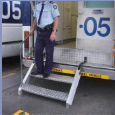
Figures 4.8 The rear of a Police “booze bus” where the well-designed access steps are stored and fold out from the rear compartment.
