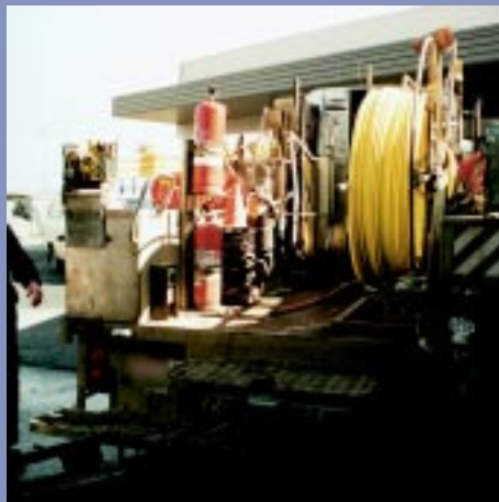
Figure 9.6 Service trucks developed for use by various utilities such as the old Gas and Fuel Corporation, incorporate good design features to increase efficiency and reduce manual handling and risk.
