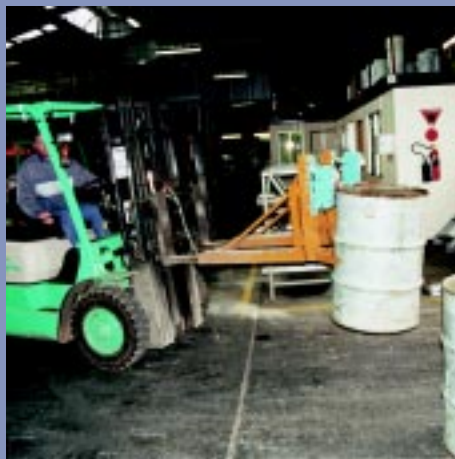
Figure 9.3 A forklift truck with drum handling attachment. It is used mainly to move full drums.
