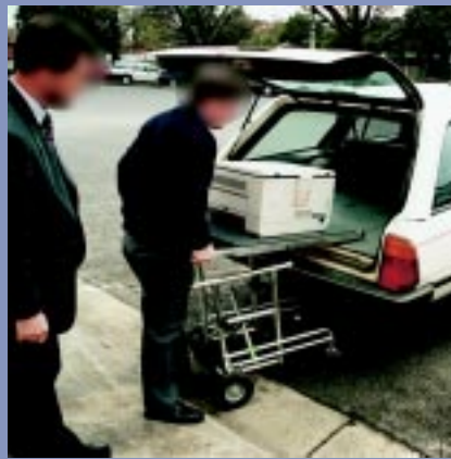
Figure 5.8(a) Use of a customised trolley for moving specific loads. This type of trolley is well-designed to suit the vehicle and particular item, thus removing the need to lift the object.
