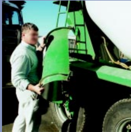
Figure 9.1 This shows the chute on a concrete truck that is made of lightweight material, replacing a heavier metal component and thereby making manual handling easier.
