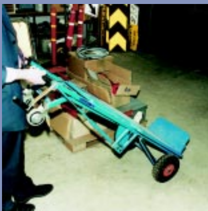
Figures 5.7(a) and (b) show a trolley that provides the option of converting to a table trolley. This is used to move loads at waist level to reducing lifting.
