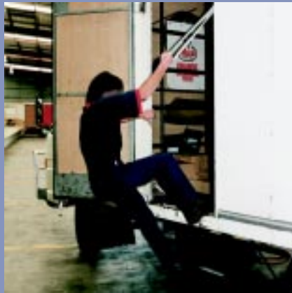
Figures 4.4 and 4.5 These photographs illustrate inadequate, but typical steps and grab handles provided for access to vans. Note the effort required to enter the doorway. Exiting is even more difficult.
