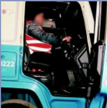
Figures 3.2 and 3.3 Examples of seating with good adjustment and support features. However, keep in mind that seating needs to be appropriate for the particular vehicle's ride characteristics and head clearance of the cabin.
