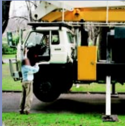
Figure 4.10 The function of the vehicle needs to be taken into account when the dimensions and design of access steps are considered: when the vehicle is in the elevated working position access to the cab is extremely difficult and risky.
