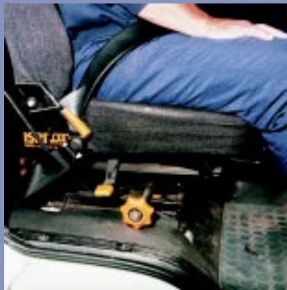
Figures 3.2 and 3.3 Examples of seating with good adjustment and support features. However, keep in mind that seating needs to be appropriate for the particular vehicle's ride characteristics and head clearance of the cabin.
