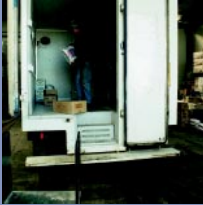
Figures 4.2 and 4.3 The rear access steps to a van, which though good in principle, are in fact hazardous due to poor design. The too narrow bottom step presents a high risk of slipping particularly whilst exiting carrying goods (wet weather would increase the slipping risk).
