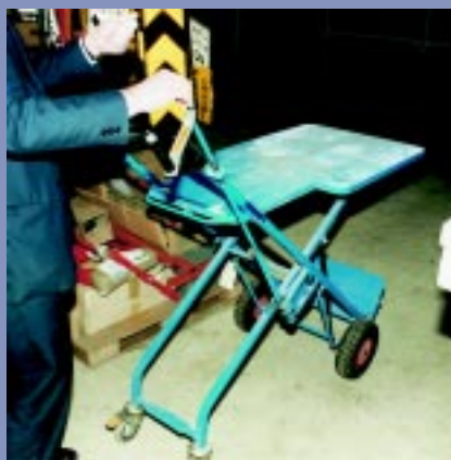
Figures 5.7(a) and (b) show a trolley that provides the option of converting to a table trolley. This is used to move loads at waist level to reducing lifting.
