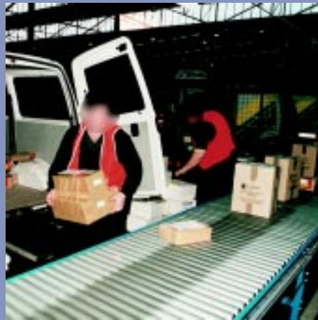
Figure 5.5 A good system for unloading from vehicles directly onto a fixed roller conveyor system (used in a freight terminal).
