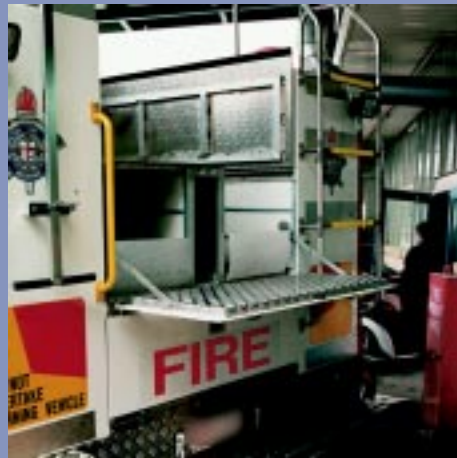
Figure 9.7(c) The rear view of the MFESB truck. Note the rear access steps and the well-designed access ladder with non-slip yellow treads. The vertical T-bar on the left side of the vehicle enables the ladder unit to be pulled down from the top of the unit, removing the need to climb on top.
