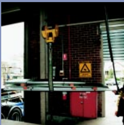
Figure 8.6 An overhead electric hoist used to unload a truck.
