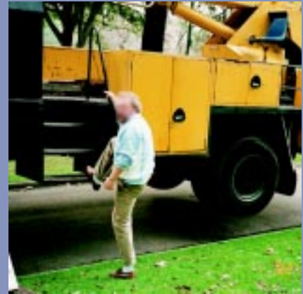
Figure 4.11 Good access steps are provided for normal operational, with the truck is in its elevated, the access points are at least 30 centimetres higher off the road, with the first step now being too high.
