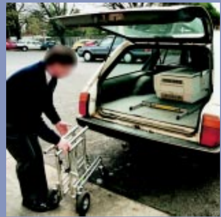
Figure 5.8(b) The trolley is lightweight, and portable, the top slides off the trolley and slides into the vehicle.
