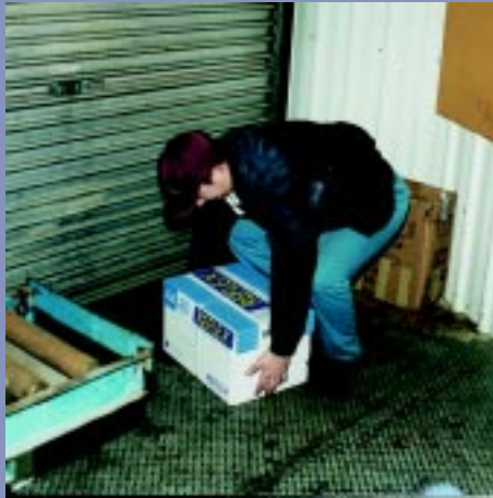
Figures 8.3 Receiving points can be forgotten areas in terms of providing adequate space and appropriate equipment. In this case the area is cramped and lacks an overhead hoist for moving heavy and awkwardly shaped items.
