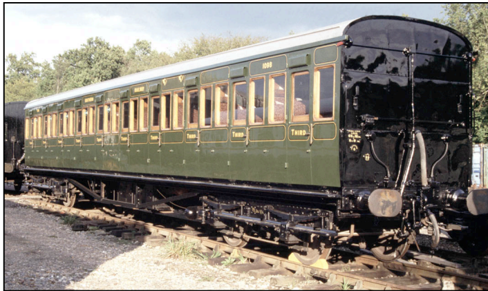
Figure 2: Typical suburban, 10 compartment coach, with seating for 100 persons, built 1922. Photo: Bluebell Railway
