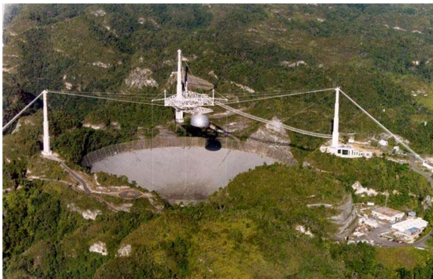
FIGURE 2.1 The Arecibo Observatory in Puerto Rico. Arecibo is used for radar observation of the Moon, Mars, Venus, Mercury, nearby asteroids, Saturn's rings, and the satellites of Jupiter and Saturn. SOURCE: Courtesy of the NAIC-Arecibo Observatory, a facility of the NSF.
